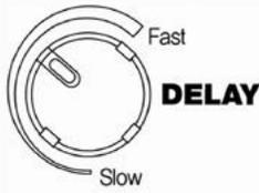
The delay functions should be used to set the recovery delay from dark to light of the welding filter according to welding method and current.
