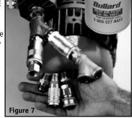
7. Before connecting your respirator to the air supply hose, turn the pump on. Allow the air to flow through the pump and hose for a few minutes to purge or expel any hose odors or moisture that may have accumulated inside the hose.
