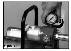
b. Remove the pressure gauge from its
