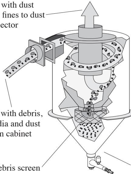
The heart of every Pulsar® cabinet is the proven ZERO reclaimer -- which efficiently separates dust and debris from reusable media. The reclaimer incorporates a wear-plate which protects the inlet from damage by debris. The large basket beneath the reclaimer screens out oversize material that can clog the blast system. A fully adjustable metering system delivers as much or as little media as needed.
