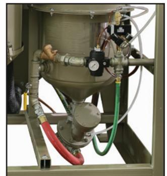
*Flange-mounted blast machine on Pulsar® VIP*
