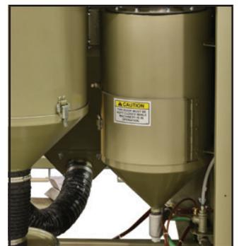
The Pulsar® suction blast cabinets combine blast, recovery, reclaim and dust collection in an efficient, compact enclosure.
