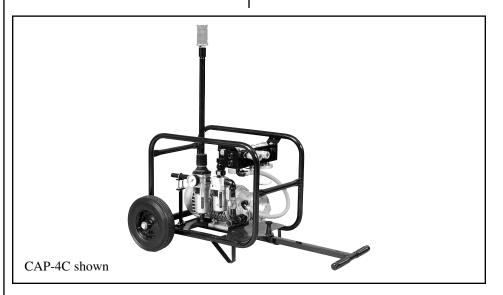
Before blasting begins, and before putting on the respirator, the operator connects the respirator hose to the ambient pump and to the fixed-orifice air inlet at the respirator. The operator starts the compressor, turns on the ambient air pump, adjusts the pressure, and checks for leaks, then puts on the respirator in a clean environment.
