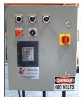
The **EVS** is able to densify the refractory without "de-airing/forking" due to the design of the variable frequency drive (control panel) and the internal weighting system of the vibrator. Operation in the **Forward** mode generates a low frequency vibration that settles the refractory. This acts as the "de-airing/forking" step. Operation in the **Reverse** mode generates a high frequency vibration that compacts the refractory to a uniform and optimum installed density.
