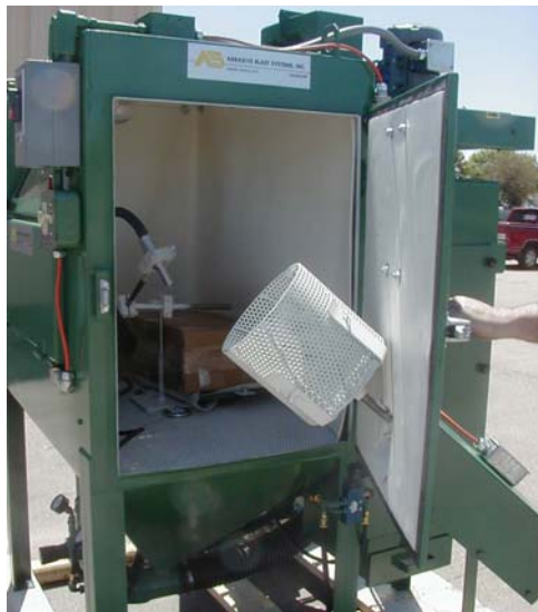
Tumble basket attachment us used for blasting small parts in a batch process. Adjustable timer and nozzle holder included.
