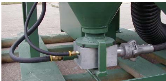
Aerated feed valves are used for extremely fine abrasives, where flowability is important.
