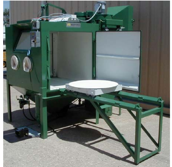
Work car and track extension make cabinet loading and unloading easy and safe.
