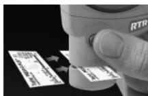
To position the tape, align the two dots (printed on replica tape) with arrows on both sides of the measurement opening.
