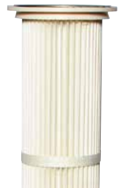
PleatPlus® IntegraSeal™ > Clean side removal > IntegraSeal fits tubesheet hole sizes from 4.625" to 8.75"
