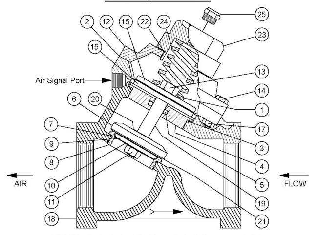
NOTE: With spring closed valve air flow is in opposite direction from arrow on valve body.
