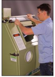
The top-mounted light module features an abrasive-resistant Lexan® cover and twin fluorescent bulbs
