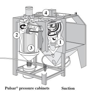
In the pressure system a 1 cu ft blast machine (5) replaces the media storage hopper. The blast machine is automatically refilled from the reclaimer (1) each time the foot pedal is released.
