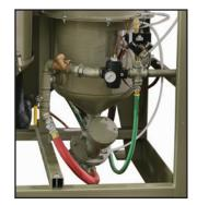
Flange-mounted blast machine on Pulsar<sup>®</sup> VIP
