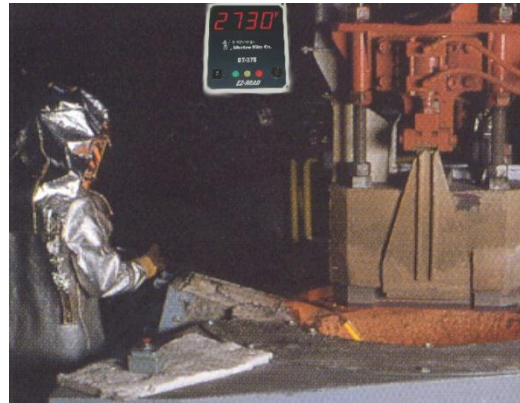
The XT E thermocouple shown measuring temperature in an induction furnace application.
