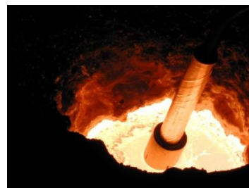
The class 3 sleeve is a custom engineered composite material that offers excellent insulation properties and durability.
